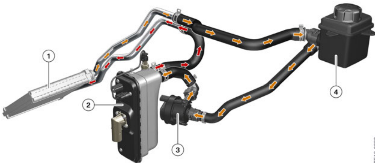
Heating for the passenger compartment in I01 with range extender
